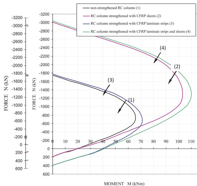
**Fig. 8** The interaction curves for all the columns tested
