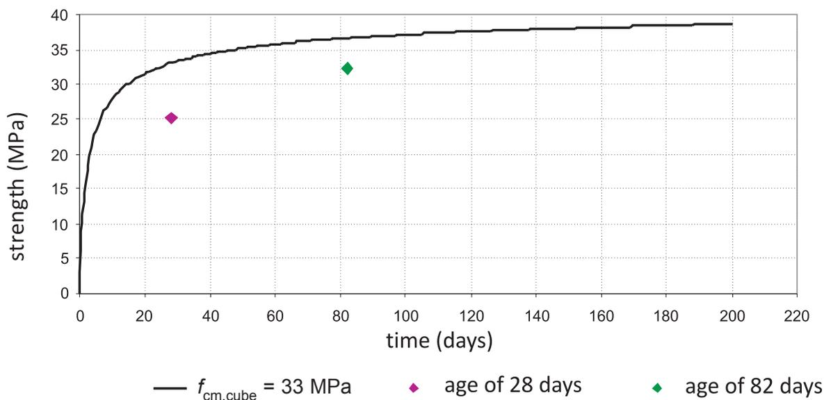
**Fig. 4** Development of the concrete's strength
