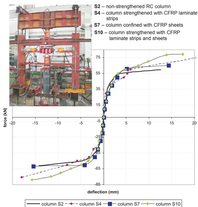
**Fig. 9** Force – deflection (LVDT1) relationship for columns, vertical load 250 kN and increasing horizontal load
