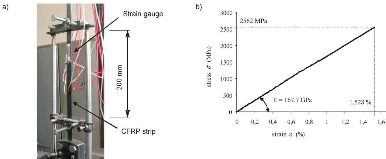
**Fig. 5** Tension test and stress – strain diagram of CFRP strip
