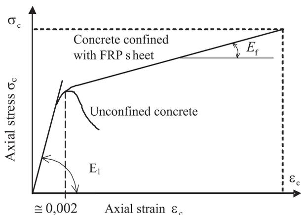
**Fig. 1** Ideal axial stress-strain diagram  $\sigma_c - \epsilon_c$  for concrete confined with a FRP sheet [6]
