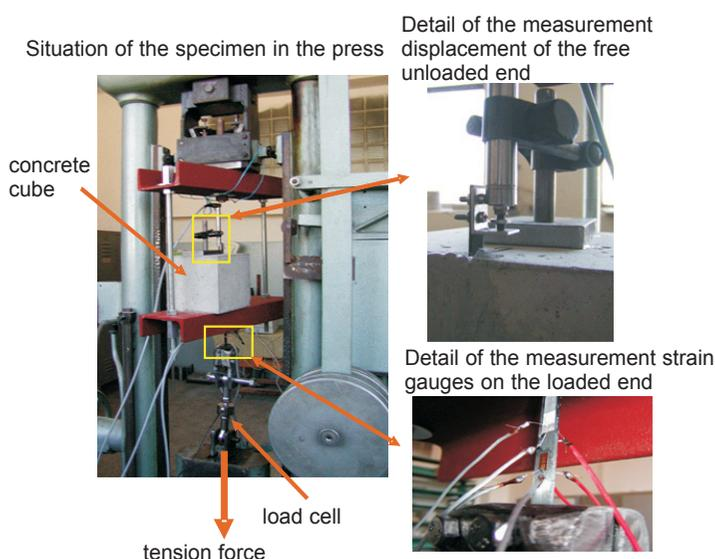
**Fig. 6** Pull-out test of the anchorage length of the CFRP strip
