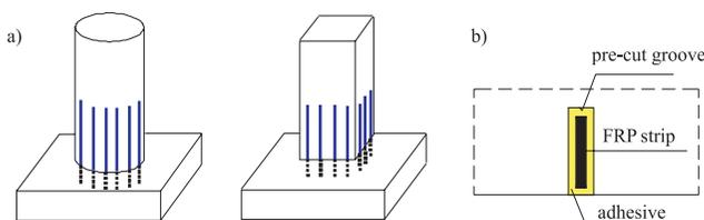
**Fig. 2a)** Technique of strengthening columns NSM FRP reinforcement [8], **b)** detail of FRP strip in pre-cut groove
