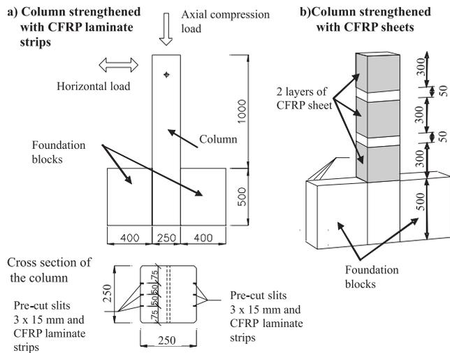
**Fig. 3** Strengthening technique adopted for reinforced concrete (RC) columns
