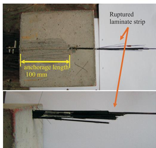
**Fig. 7** Pull-out test of the laminate strip inserted in a groove in the concrete fragment
