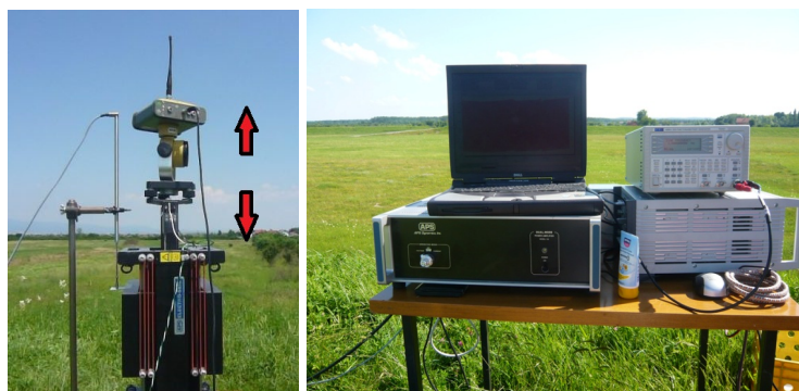
Figure 1 Electrodynamic oscillator with mounted circular prism and GNSS (a), frequency generator with amplifier (b)
