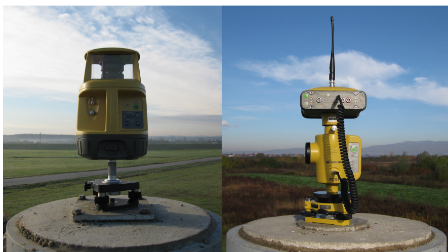
Figure 1 (a) PZL-1 laser transmitter and (b) PZS-1 sensor connected to GNSS rover receiver
