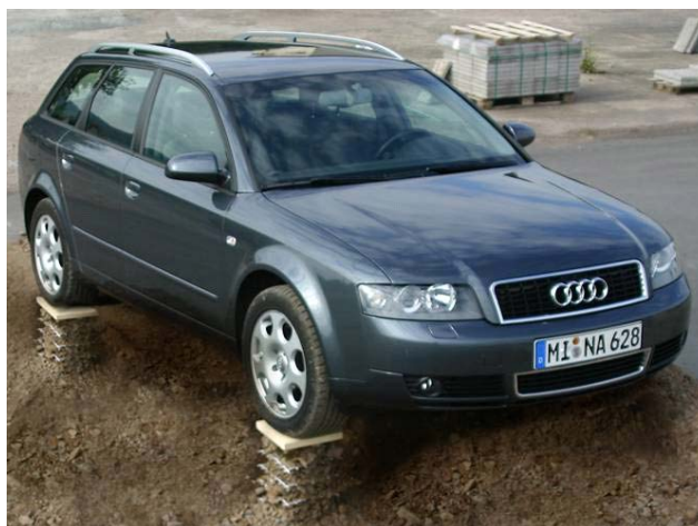
Fig. 1. Geogrid reinforced gravel columns carrying a car
