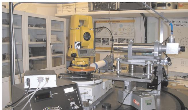
Fig. 3 Calibration of Topcon GTS 6B instrument on the EZB – 3
