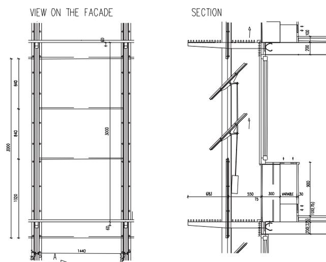
**Fig. 1** Section of solar double-skinned facade with opening louvers and internal and external open grate walkways on the Moravian Regional Library in Brno
