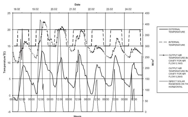
**Fig. 5** Simulation of air temperatures in the cavity of double solar facade preheated from direct radiation for two steady forced air flows 0.1 and 0.2 m.s-1. Climate output data are used from TRY (station Kucharovice, CZ)
