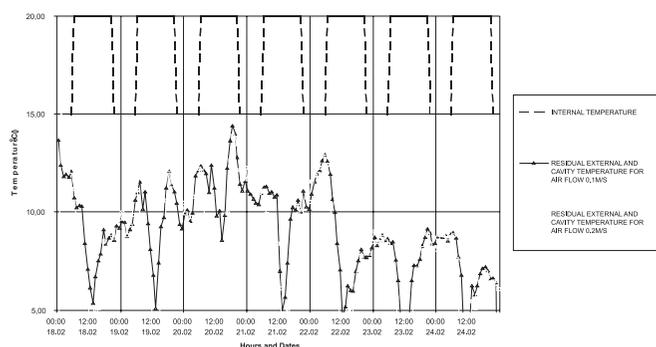
**Fig. 6** Residuals of external and cavity output temperature simulated for air flow velocity 0,1 m/s and 0,2 m/s in the convection channel of the solar facade in the recovery period
