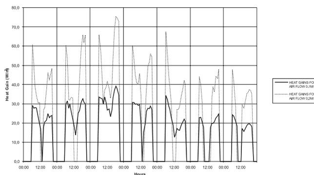
**Fig. 7** Simulation of heat gains from solar preheated air in the facade used for heating in ventilation system
