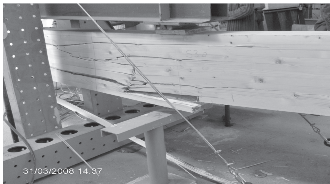
Fig. 6: Failed beam with loosened load-carrying capacity (Beam №3)
