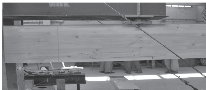
Fig. 5: First cracks of the beam (Beam №3)
