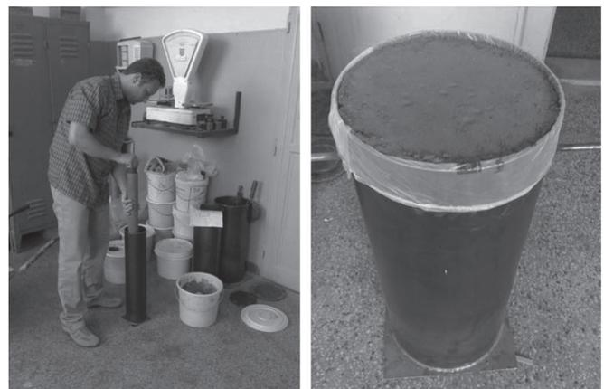
**Fig. 1** Compacting of soil prepared for the formation of the stone columns.
