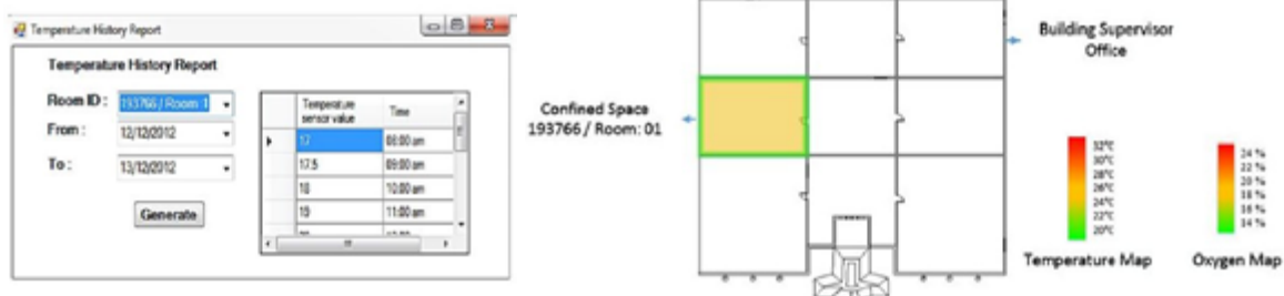
Figure 3– Temperature history report. Figure 4 - Different surface and boundary color shows different status of sensor readings (temperature, oxygen) in confined space. [3]
