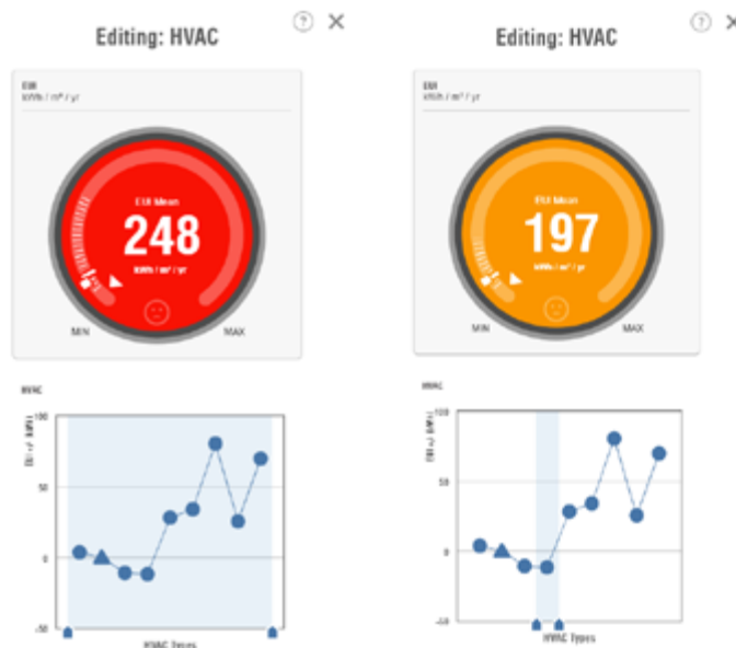
Figure 4 Showcase of an automatic calculation and of EUI in Insight tool when manually adjusting design parameters during conceptional design stage
