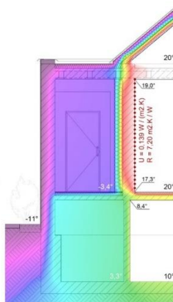
Variant A Full roof, non-transparent vertical constructions
