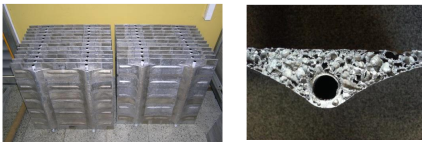
Fig. 5.2 The radiant panel with pipes in foam aluminium
