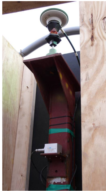
Figure 4 Collocated Active Prism and inclinometer (Whitworth, 2010)
