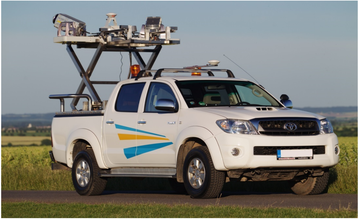
Figure 1 Surveying vehicle with LYNX M1 and POS LV 520
