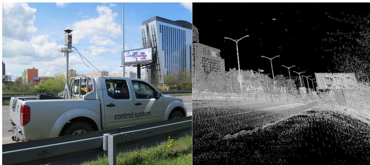
Figure 1 3D TLS – technology of the precise measurement of the road surface
