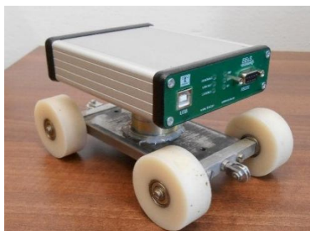
Figure 5 IMU EEaS placed on cart
