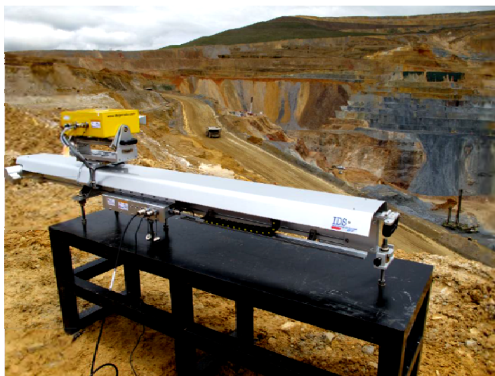
Figure 2 The IBIS-L ground based radar system in front of an open-pit mining area. The radar head moves on a 2m long rail and is oriented towards the critical slope (IDS)
