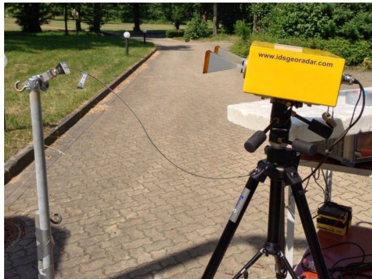
Figure 7 Frequency check for IBIS-L: The antenna of a spectral analyzer is positioned outside the radar head.
