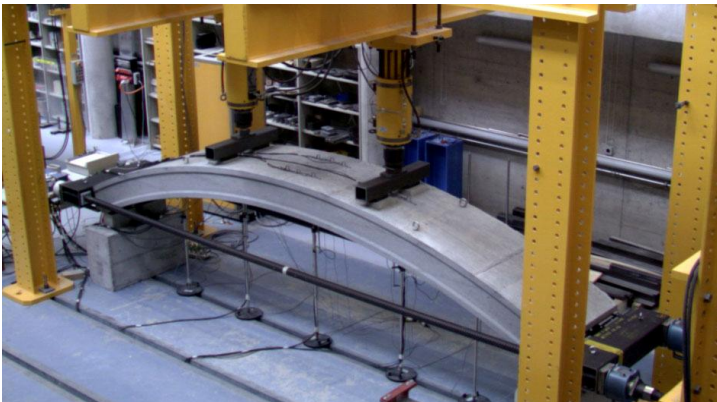
Figure 8: Full scale load tests on precast tunnel segment
