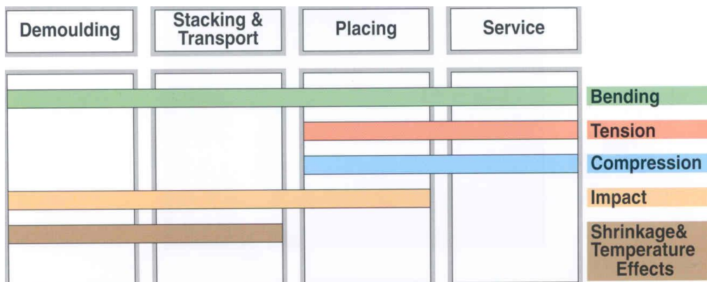
Figure 3: Illustration of the acting loads on segments
