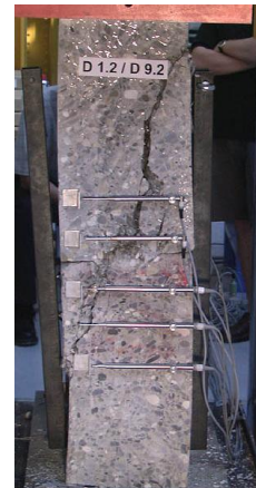
Figure 10: Tests set-up on joint connections between segments
