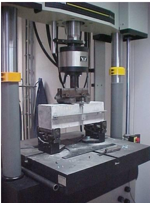
Figure 5: Four point bending test beam
