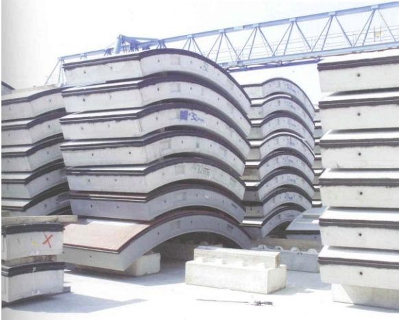
Figure 1: Stacking of segments
