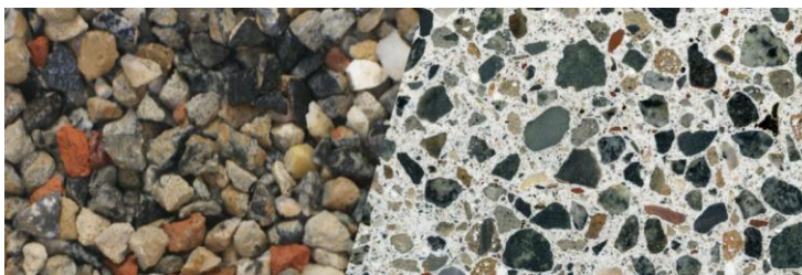
Figure 1: Cross section of concrete on recycled aggregate
